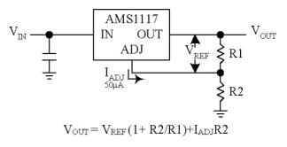
Figure 2. Basic Adjustable Regulator
